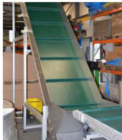
INCLINED BELT CONVEYOR
